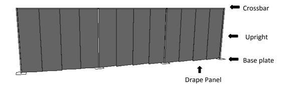
Always check if the set-up is going to be 2 or more separate sections or all connected in 1 long line, even if there is a 90 degree bend in the line. It often helps to draw it out and then count the parts.
